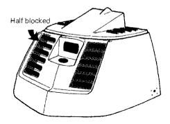
When operating the vehicle in powder snow it is advisable to block the front cab louvers as per illustration. Unblock the louvers as soon as snow condition becomes firmer or as soon as engine becomes too hot.
