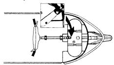
Grease the ski leg at grease fitting until new grease appears at the joint. Lubricate spring coupler bolt with oil.
