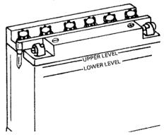
If necessary add distilled water. Battery connections must also be free of corrosion. If cleaning is necessary, remove corrosion using a stiff brush then clean with a solution of baking soda and water. Rinse and dry well.
