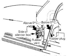
In temperatures below 0° C (32° F) and/or powder snow, the rubber plug must block the entry of fresh air on the side of the silencer box and the rubber vent must allow the warm air being emitted from the engine to be directed over the carburetor.
