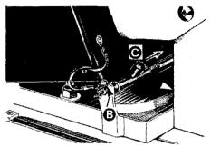
3. Move pulley guard toward front of vehicle to disengage front attaching device from front bracket.
